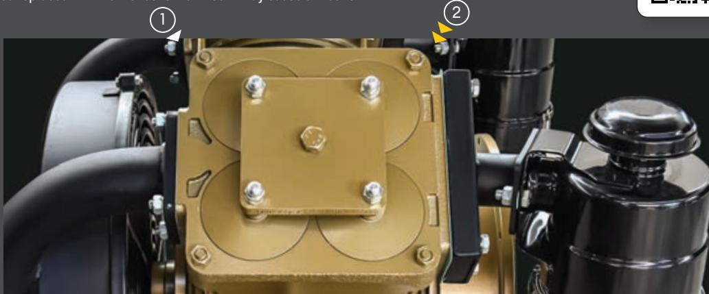
Air intake block nuts must be tightened to 5 kg. The removed nuts must be tightened diagonally.
